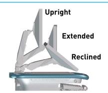
Monitor Rotation  $80^{\circ}$  left or right (remove the rotation limiter pin to rotate fully to the right)
